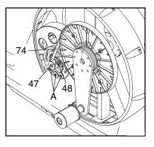
of the elliptical exerciser until the Belt (74) is tight. Then, tighten the three screws.
